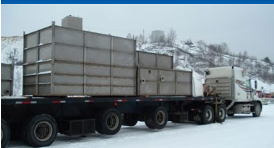
Biowater package plant loaded on a trailer for transportation.
