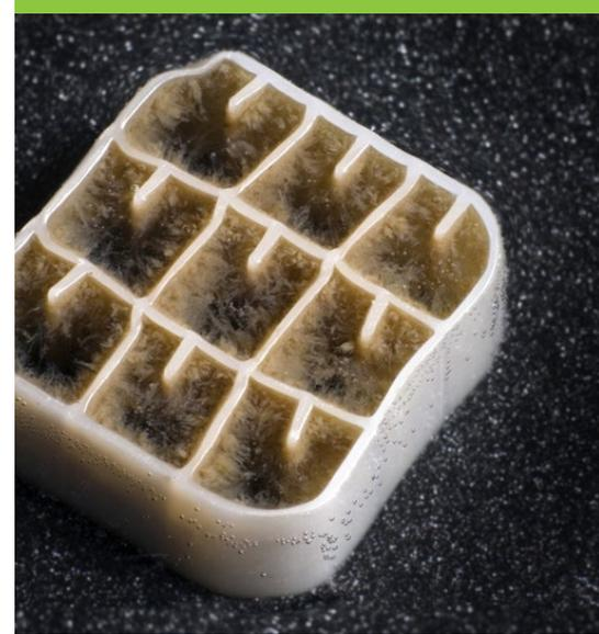
*The basis of our CFAS® biofilm technology is the biological growth on polyethylene pieces called media or carriers. These surfaces provide a protective surface area for the biology to grow. The biofilm can handle extremely high loading conditions without any problems with clogging or shock.*
