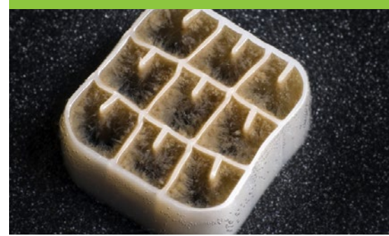
The BioWater CMFF® biological process is based on the MBBR (Moving Bed Bio Reactor) concept where moving plastic carriers with fixed biofilm remove organic and inorganic substances in the water. The proposed BioWater CMFF® design includes the Biowater biofilm carrier elements which are freely mixing around in the reactor and are specially designed for biofilm growth.
