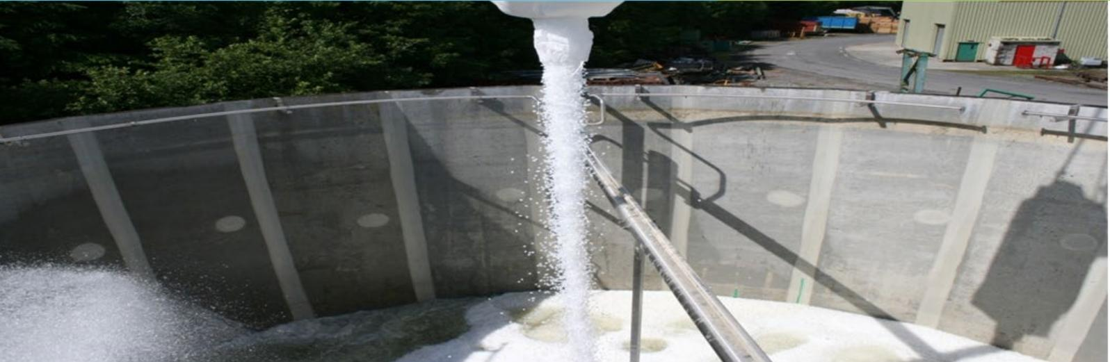
*Bioreactor being filled with media.*
