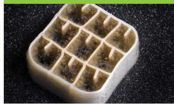
The basis of our CFAS® biofilm technology is the biological growth on polyethylene pieces called media or carriers. These surfaces provide a protective surface area for the biology to grow. The biofilm can handle extremely high loading conditions without any problems with clogging or shock.
